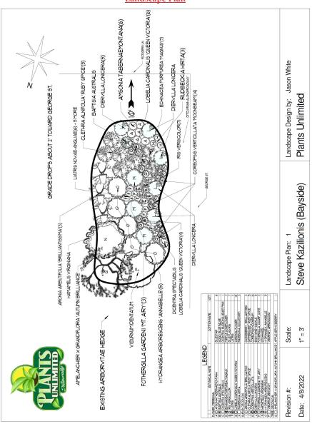
Note: The orientation of the compass rose on this landscape plan is incorrect. Its orientation is off by 180 degrees.
